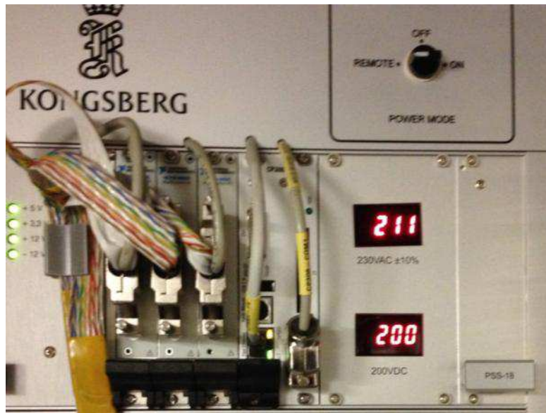
Figure 13 Input AC voltage meter (top) in TOPAS transceiver.
