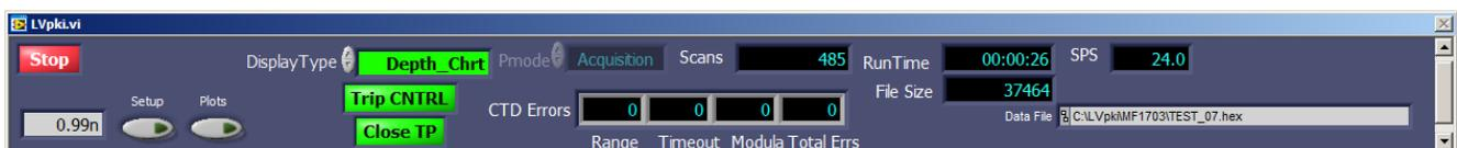
On the upper left panel, GPS data should be displaying. Near the bottom of the panel the Net Angle indicator should be seen. There are two green warning indicators that will flash red if there is a problem with either the CTD or NMEA signals. Latitude and Longitude can be displayed in either traditional or decimal format by clicking on the DegMin or Decimal button
